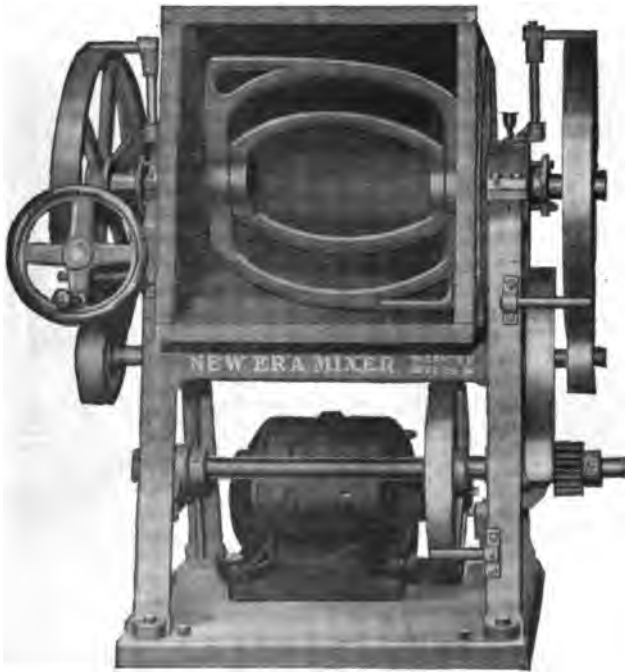
FIG. 11.—Bread mixer. American Oven and Machine Co., Chicago.
